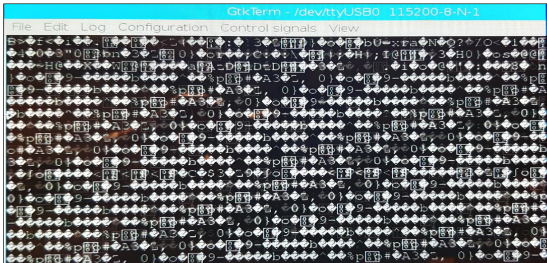
Figure 30: The junk character data logged as the output from the Ellipse2-D in the RevPi Compact with GTK Terminal.
