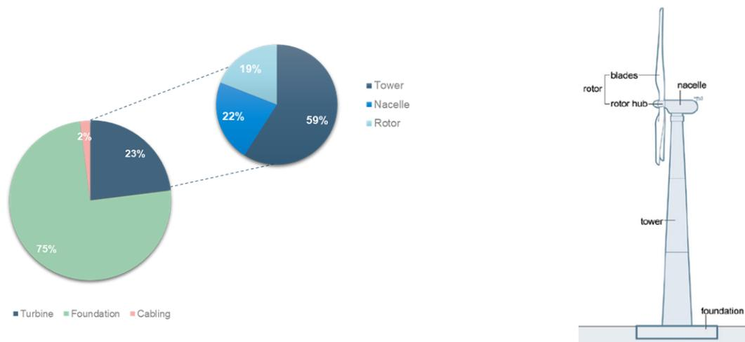
Figure 2: Composition of wind turbines (average onshore and offshore)
