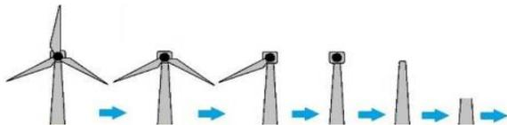
Figure 4: Reverse installation method
