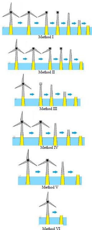
Figure 5: Decommissioning techniques offshore wind turbine
