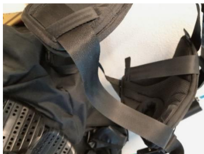
Figure 3: straps at the bottom of the side cuffs (similar to Laevo Flex)
