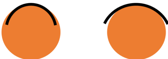
Figure 3: Fit of a small radius cuff (black) vs. large radius cuff around leg (orange)
