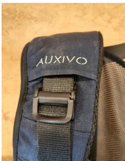
Figure 2: Strap anchor tends to slide
