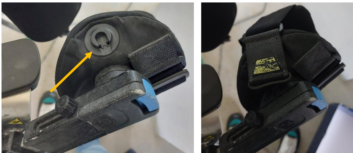
Figure 1. The lock system of the arm cuffs strap, with the strap open and closed.
