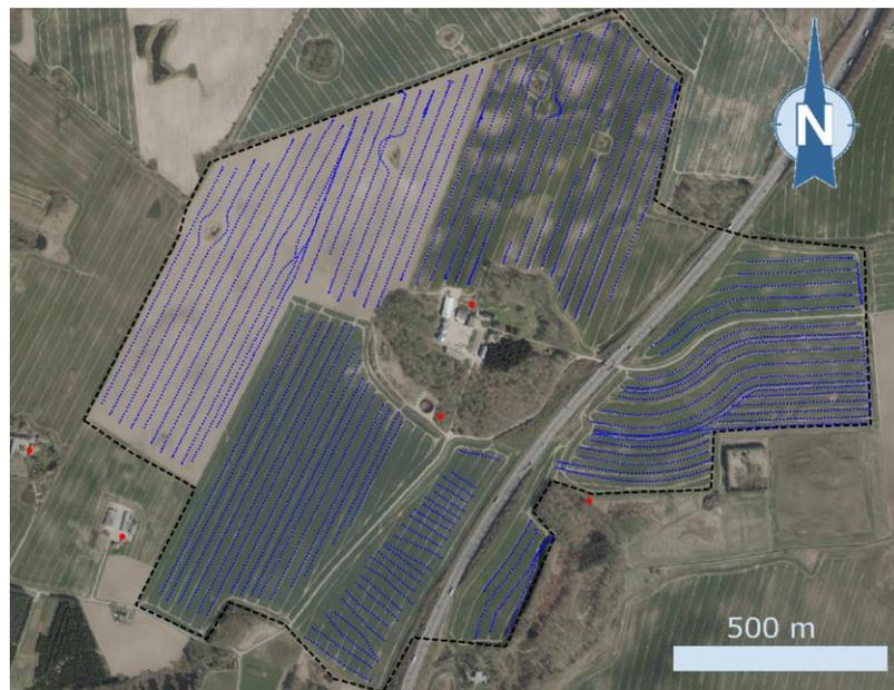
Figure 1. Survey area, with tTEM lines in black. Each blue dot corresponds to one tTEM sounding/resistivity model. The model spacing along the lines is ~15-25 m. The red circles shows boreholes in the area.
