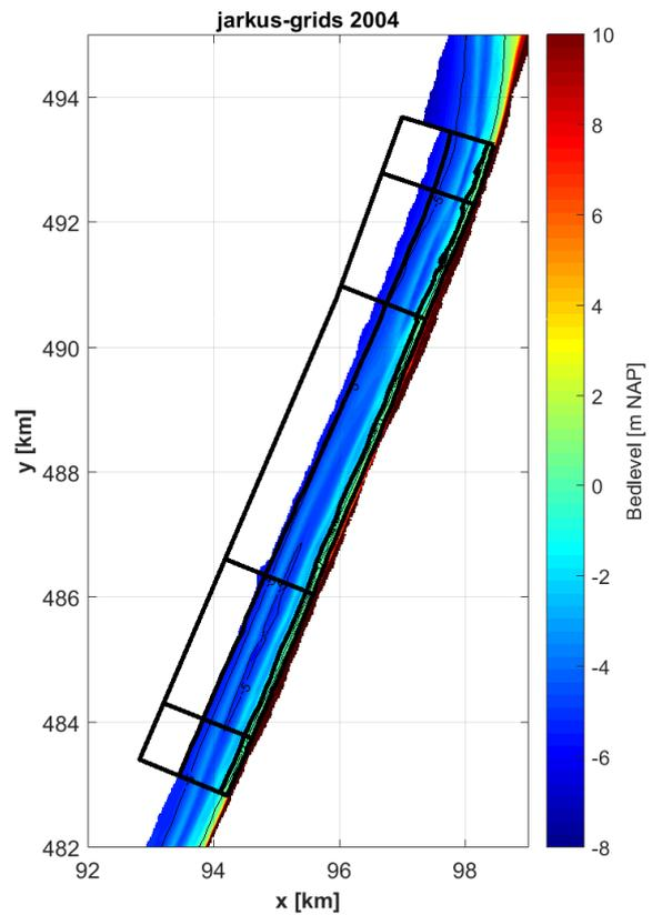
Figure 10: A top view of the bathymetry in 2004 based on Jarkus-grids. The black squares indicate different areas which will be used in Section 6.2.
