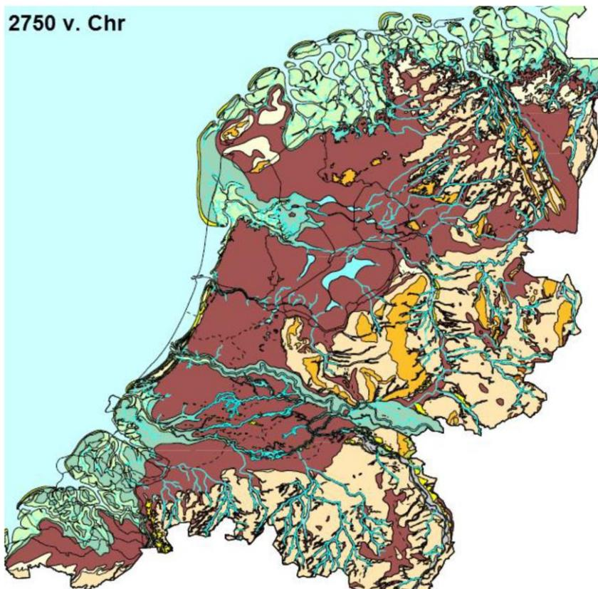
Figure 2: The different areas of the Netherland 2750 v. Chr. The yellow part indicate sand, the brown is peat and the green areas are partly submerged regions for example because of the tides. The thin black line indicate the current location of the Dutch coast.
