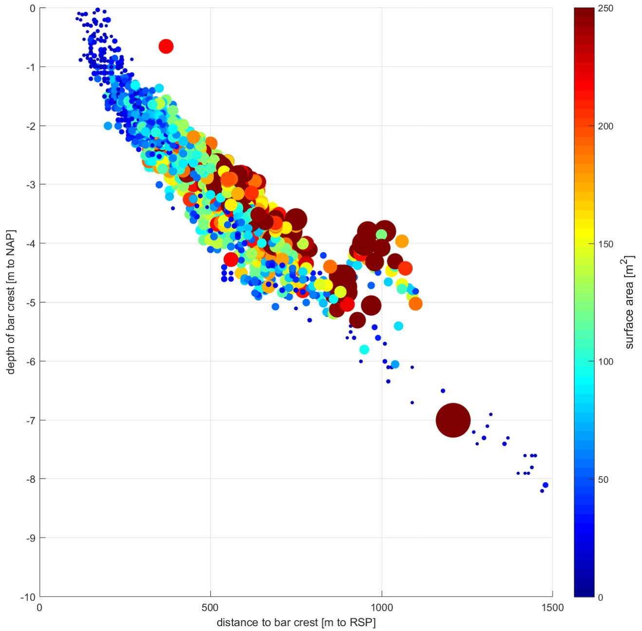
Figure 47: Relation between horizontal distance to bar crest and depth of the bar crest, for each bar in all measured years. Colours and circle-size correspond with surface area of the bar (m<sup>2</sup>)
