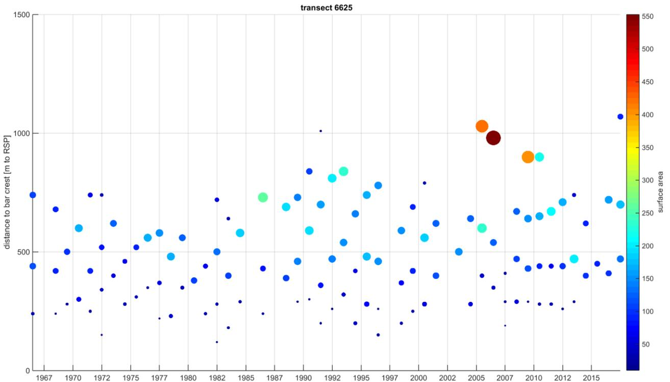
Figure 49: Development of bar crests position over time for transect 6625, colours and circle-size correspond with surface area of the bar ( $m^2$ ), dashed arrows indicate movement of single bar in time. The nourishment is clearly visible in 2005 by its larger surface area and far offshore position.
