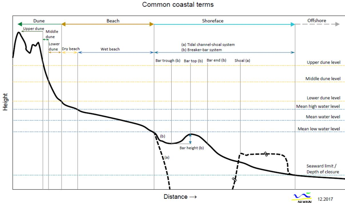
Figure 14: General definition/terminology coastal profile used. On the vertical axis various levels in the profile are shown. The horizontal axis shows different zones in the profile. Source: Simon Hillmann (NLWKN)
