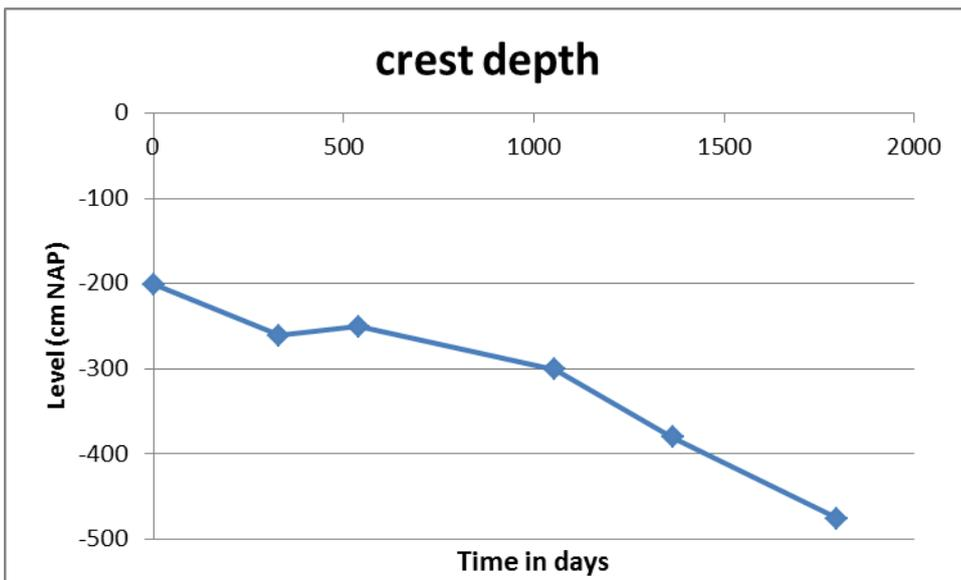
Figure 46: Change of crest depth in time for a randomly chosen bar (same bar as in Figure 44)
