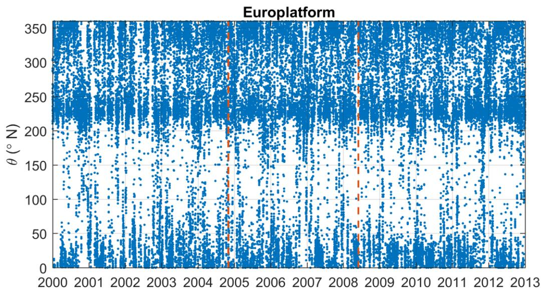
Figure 19: The measured value of  $\theta$  at the Europlatform. The red dotted lines indicate the nourishments.
