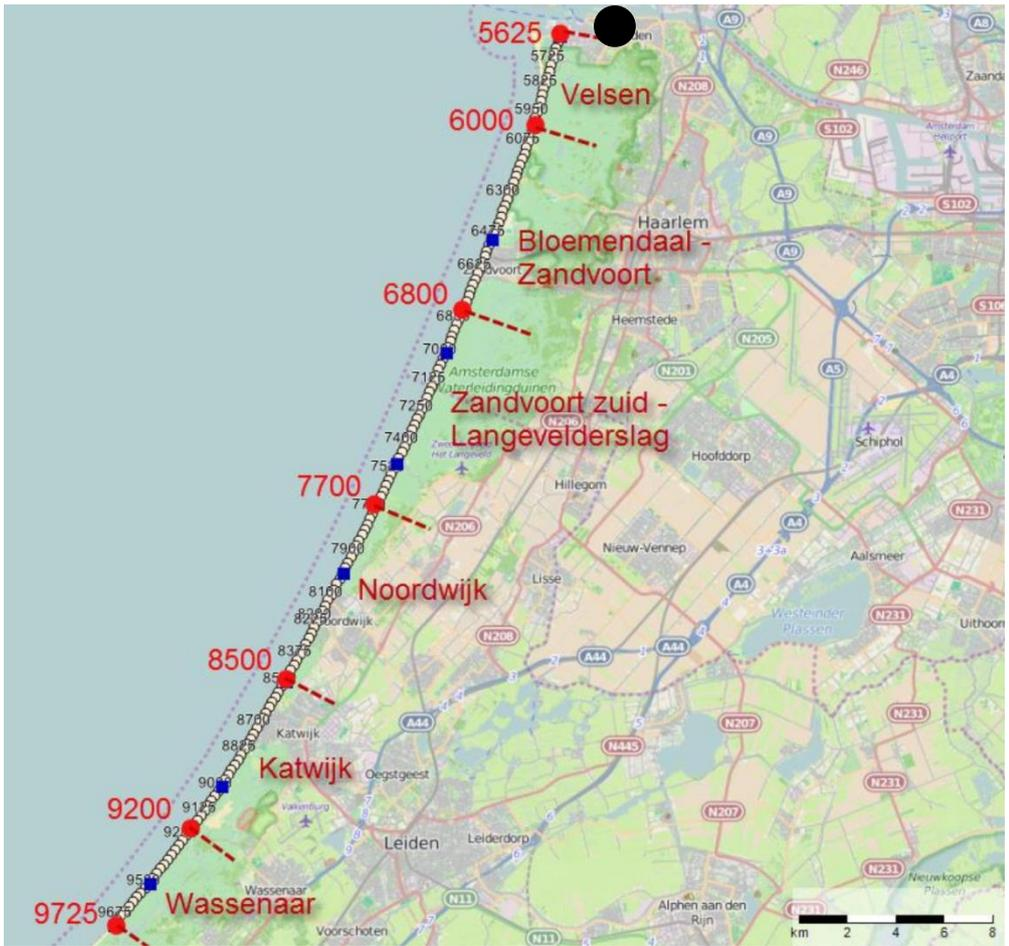
Figure 5: A map of the area around Zandvoort-Bloemendaal. The numbers indicate the different Jarkus transects. The black dot indicates IJmuiden where large breakwaters and sluices are located. Adjusted from (Kuijper, Nederhoff, & Vergouwen, 2015)
