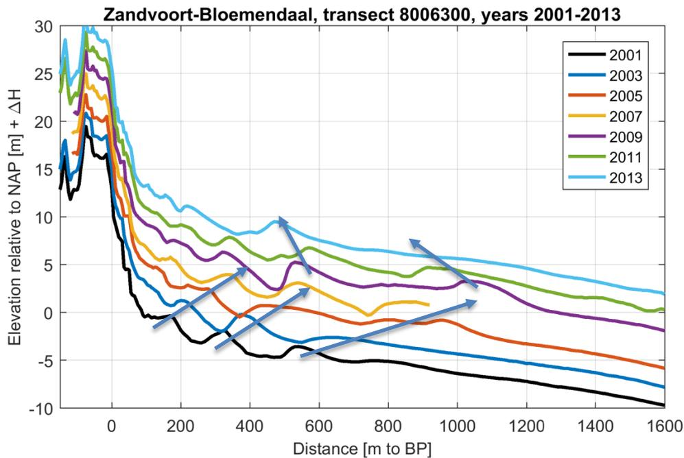
Figure 29: A plot of the bathymetry measurements for Jarkus transect 6300. The bathymetry is manually shifted up using a  $\Delta H = 2\text{m}$  for each line. The arrows indicate the movement of the bars.
