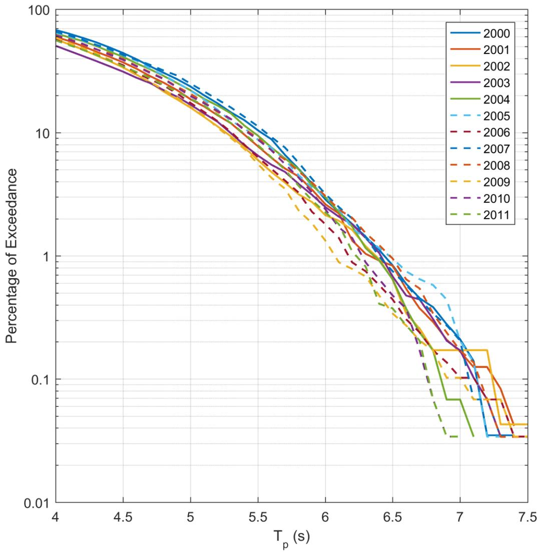
Figure 22: Percentage of exceedance of the measurements for  $T_p$  at the Europlatform for each year.
