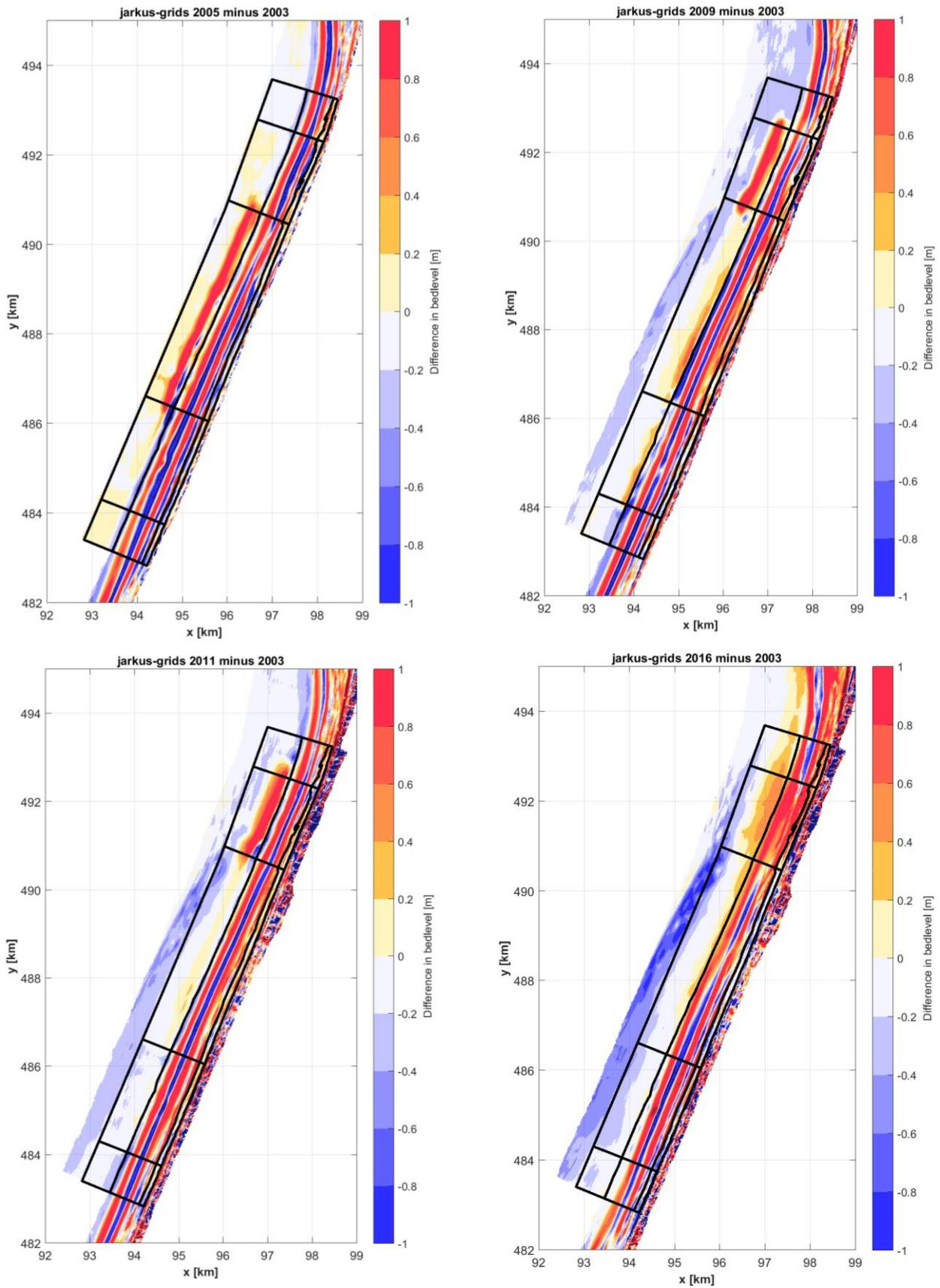
Figure 53: The difference in height between different Jarkus grid. The difference are calculated compared to the year of reference 2003.
